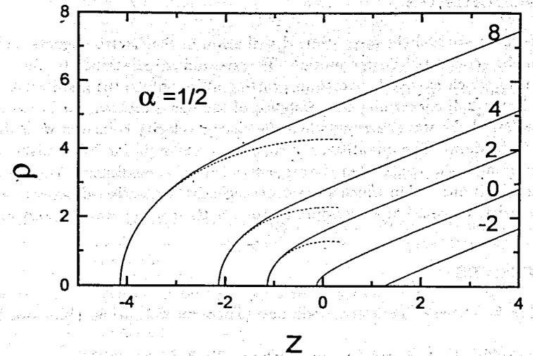
Fig.7: Continuous transformation of the Cherenkov shock wave attached to a moving charge ( $t = -2$ ) into the blunt shock waves ( $t = 2, 4, 8$ ) detached from a charge for the decelerated motion and  $\alpha = 1/2$ . The charge motion terminates at the moment  $t = 0$ . The numbers near the curves mean the observation times. Short dash curves are the same as in Fig. 5.
