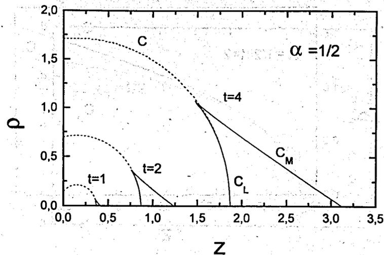
Fig. 3: Time evolution of the shock waves for the uniformly accelerated charge and  $\alpha = 1/2$ .  $C_M$  is the usual Cherenkov shock wave,  $C_L$  is the shock wave emitted at the moment when the charge velocity coincides with the medium light velocity. Short dash curves  $C$  are the same as in Fig. 1.
