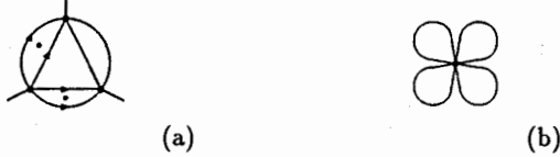
Figure 1: The divergent four-loop momentum integrals in the N=2 supersymmetric two-dimensional \sigma model. Lines represent 1/p^2 propagators, arrows stand for additional p_\mu in the numerator, and small dots denote contractions of Lorentz indices.
