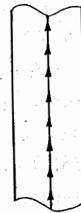
Fig.3. The explicit realization of magnetic (electric) cylindrical solenoid by means of linear magnetic (electric) dipole chain.
