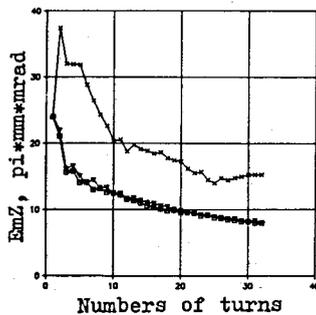
Fig. 2. Effective emittance of the axial motion as a function of the turn number. 1 - 0.3 mA, 2 - 8 mA,  $E_r = 20\pi$  mm mrad; 3 - 8 mA,  $E_r = 40\pi$  mm mrad.
