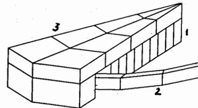
Fig.1. General view of the magnet. 1 - sector shim, 2 - winding, 3 - yoke.
