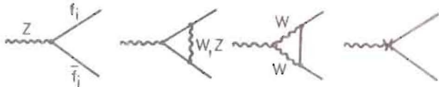
Fig.1. Born and one-loop electroweak contributions in the unitary gauge to the partial width \Gamma_i^{\text{ew}} of the decay Z \rightarrow \bar{f}_i f_i .
