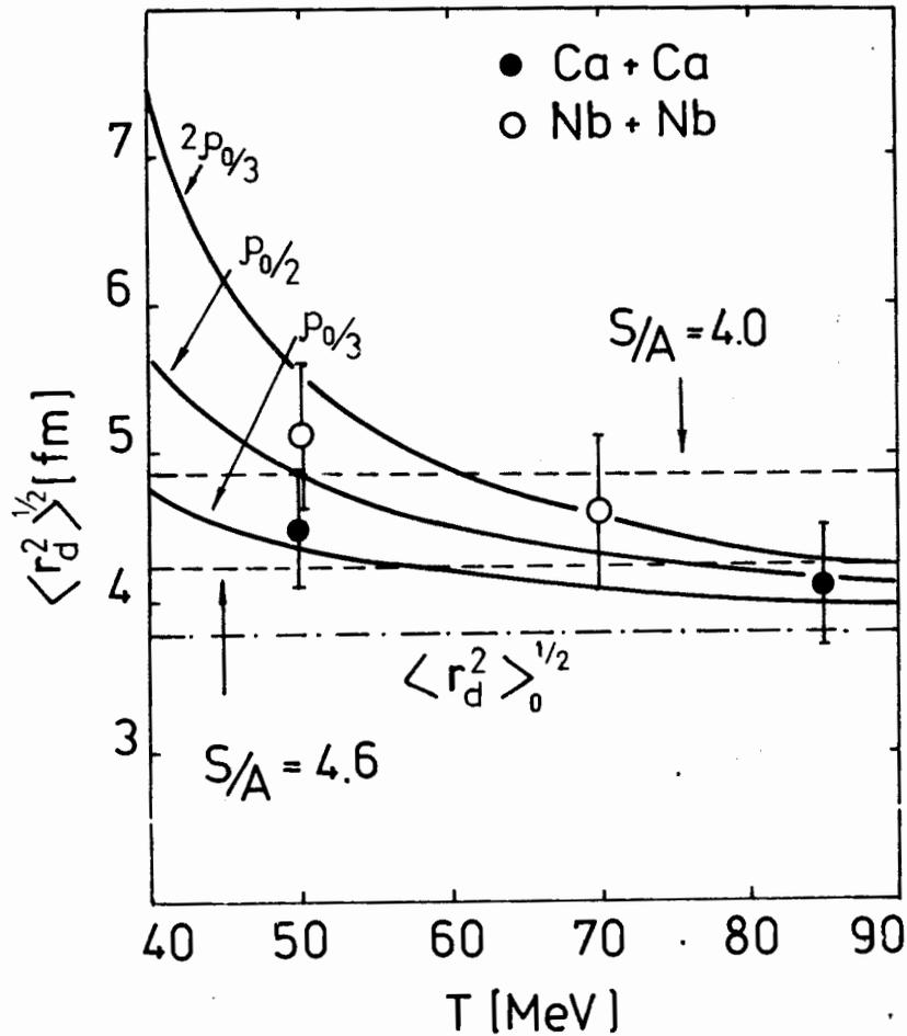
The effective deuteron radius as a function of the temperature for given break-up density (solid lines) and the given entropy value (dashed lines). The dash-dotted line indicates the rms radius of a free deuteron. The experimental points are from Doss et al.<sup>2/</sup> The specific entropy values vary between 4.0 and 4.2 when taking their fitted break-up density values and calculating the entropy values with the free Fermi gas formula.
