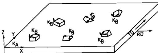
Fig. 1. The sample fixed coordinate system  $K_A$  and the crystal fixed coordinate system  $K_B$ .
