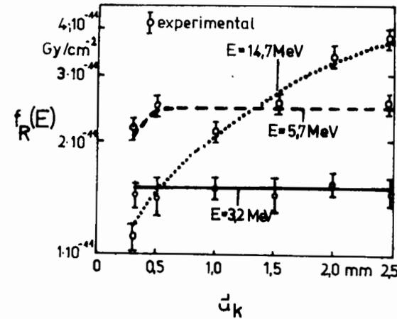
Fig.3. Dependency of the sensitivity component  $f_R(E)$  on the contact radiator thickness  $d_k$
