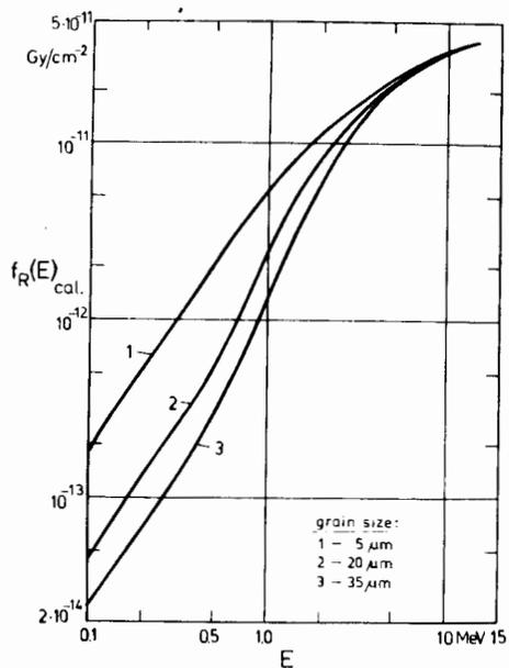
Fig.5. The influence of different grain sizes on the neutron sensitivity component  $f_R(E)$ .
