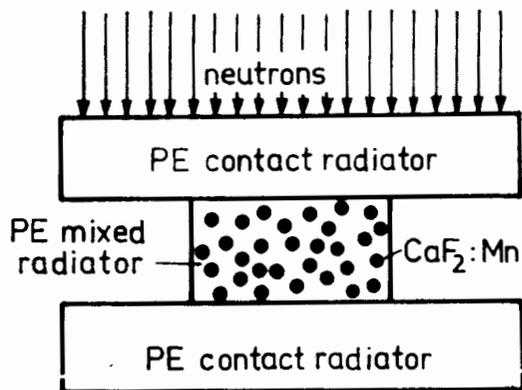
Fig.1. Detector-radiator combination (schematic).
