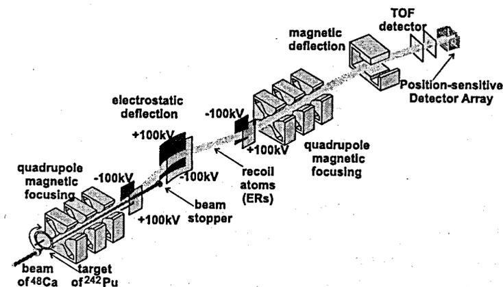
Figure 1: The schematic view of the separator VASSILISSA.
