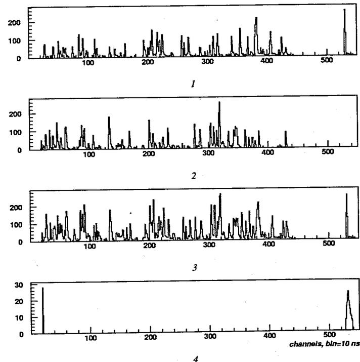
Figure 2: FADC signals for a single muon. The signals are shown for ND1 (1), ND2 (2) ND1 and ND2 together (3) and for the muon and electron detectors (4)
