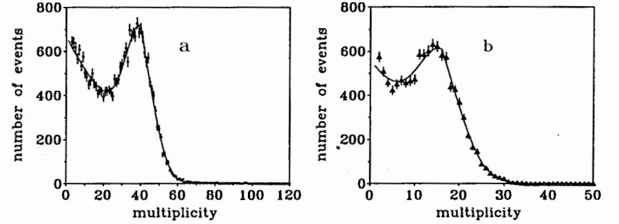
Figure 3: Neutron multiplicity distributions. Spectrum "a" corresponds to the exposure with  $C_T = 35.8\%$  and was plotted for both ND and time interval  $T = 1 \mu s$ . Variant "b" was selected for  $C_T = 88.5\%$ , both ND and  $T = 2 \mu s$ . Curves are the optimum fits.
