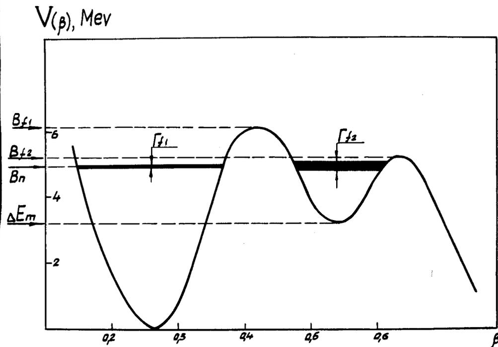
Fig.3. Potential energy ( $V$ ) as a function of nuclear deformation ( $\beta$ )
