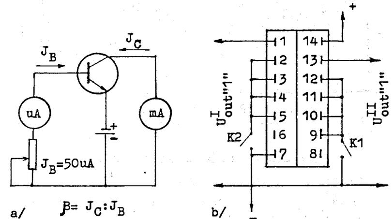
Fig. 2. Measuring systems: a) for the dc gain of bipolar transistors -  $\beta$ , b) for output voltage of NAND gates -  $U_{\text{out}}$ .
