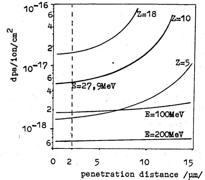
Fig. 1. Atom displacements density on the penetration distance in Si for different Z and E of incident ions. Theoretical curves.
