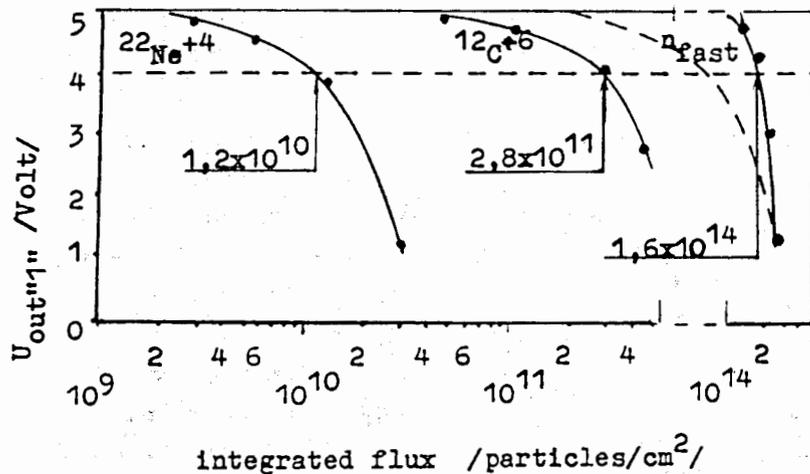
Fig.4. MCA 54012 NAND gate degradation of output voltage for logical state "1" vs incident ion flux. Ion parameters: Ne - 27.9 MeV, C - 91 MeV.
