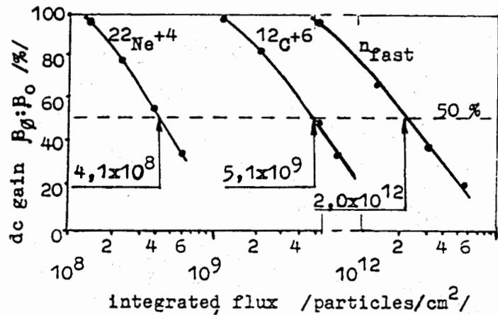
Fig.3. BC 177 transistors gain degradation vs incident ion flux. Ion parameters: Ne - 27.9 MeV, C - 91 MeV.
