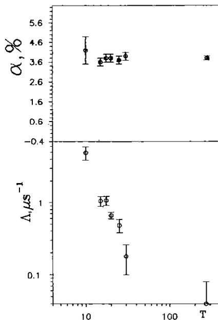
Fig. 2. Asymmetry coefficient  $\alpha$  of the  $\mu^- \rightarrow e$  decay electrons and muon spin relaxation rate  $\Lambda$  as a function of temperature in Si.
