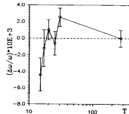
Fig. 3. Paramagnetic shift of the muon spin precession frequency in Si as a function of temperature.
