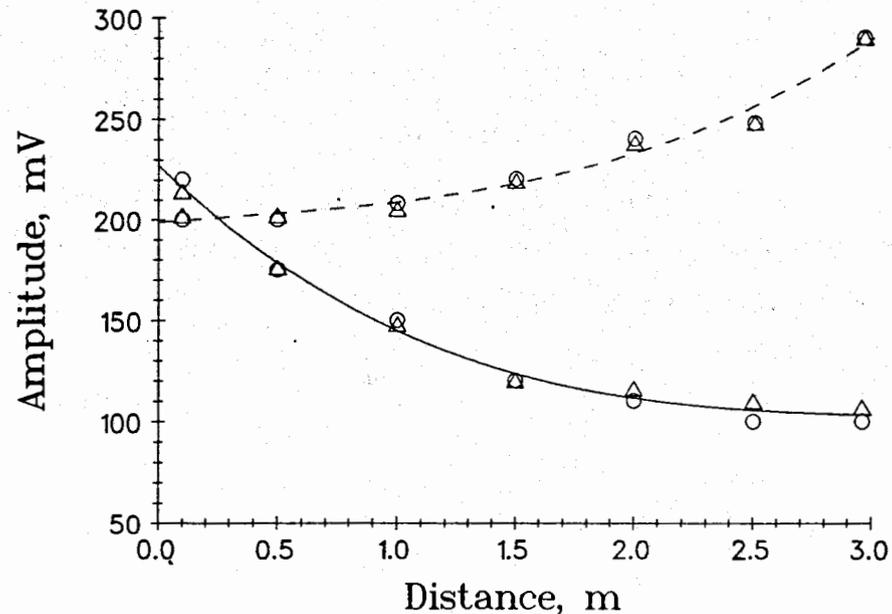
Fig. 4 Ratio of anode amplitudes vs the position of the  $^{55}\text{Fe}$  source along the straw. Solid curves represent the terminated straws ( $R = 230 \text{ Ohm}$ ), dashed curves represent the non terminated straws ( $R = \infty$ ). Width of the strips is 8 mm,  $R_{str}$  is  $3.1 \text{ Ohm} / \text{mm}^2$ .
