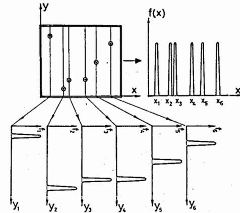
Fig. 7. Example of six vertical particle tracks shown as  $\odot$  inside the square to be scanned (see text).
