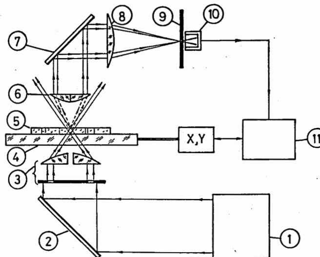
Fig. 6. Complete scheme of the new confocal microscope for selective observation of the vertical particle tracks with convergent and divergent geometries of the light rays in the illuminating and imaging objectives: 1 — laser, 2 — plane mirror, 3 — cylindrical interference illuminated system, 4, 5 — nuclear emulsion layer with vertical particle tracks, 6 — cylindrical interference imaging system, 7 — plane mirror, 8 — lens, 9 — pinhole, 10 — photodetector, 11 — computer.
