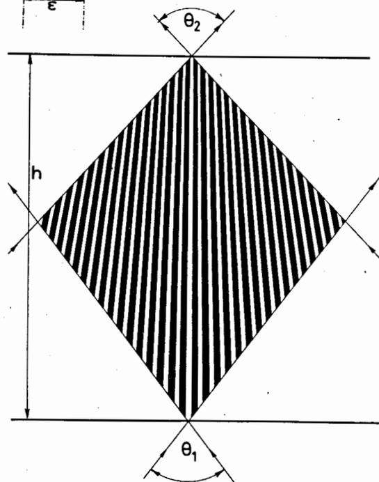
Fig. 2. Microscopic pattern of the interference picture produced by two restricted convergent cylindrical waves:  $\theta_1$  and  $\theta_2$  are the angles between two wavevectors at the upper and at the bottom surfaces of the nuclear emulsion layer, respectively.
