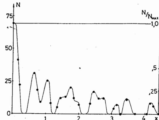
Fig. 5. The tabulated response of the confocal system with convergent and divergent objectives for vertical particle track with 75 silver grains in the nuclear emulsion layer of the depth 200  $\mu\text{m}$ .
