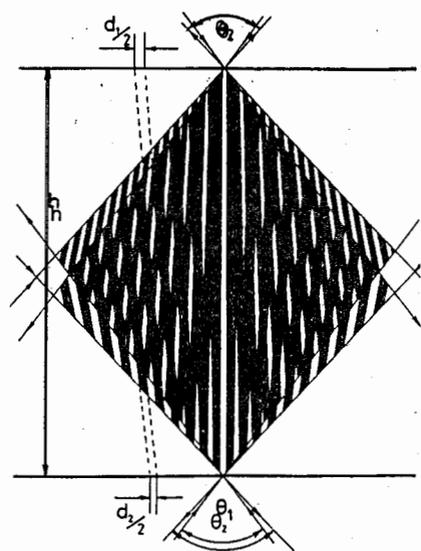
Fig. 4. An example of the overlapping pattern produced by the device with convergent cylindrical illuminating objective and with divergent cylindrical imaging objective.
