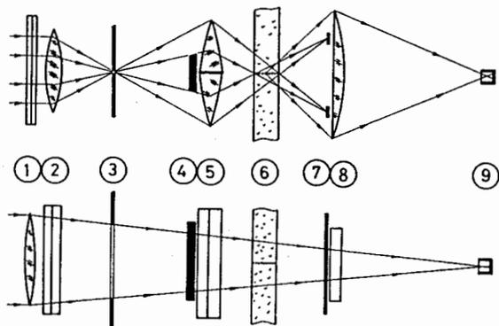
Fig. 3. Microscope for selective observation of the vertical particle tracks with convergent cylindrical illuminating light beams: 1 — first cylindrical lens, 2 — second cylindrical lens, 3 — 1D pinhole, 4 — stop, 5 — cylindrical half-lenses, 6 — nuclear emulsion layer, 7 — 1D stops, 8 — cylindrical lens, 9 — photodetector.
