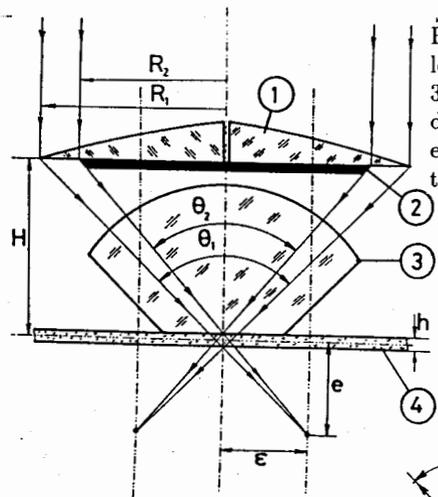
Fig. 1. Meso-optical condenser with immersion lens: 1 — cylindrical half-lens, 2 — central stop, 3 — immersion lens with enter surface perpendicular to the incoming light rays, 4 — nuclear emulsion layer,  $\epsilon$  — transversal eccentricity of the half-henses,  $(H + e)$  — its focal length.
