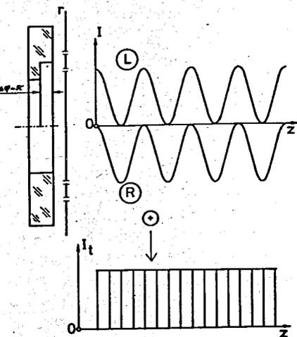
Fig. 7. The formation of the longitudinal interferences in two halves of the filter in the system with two coaxial narrow transmitting rings on the screen and the sum of these pictures on the optical axis of the system.
