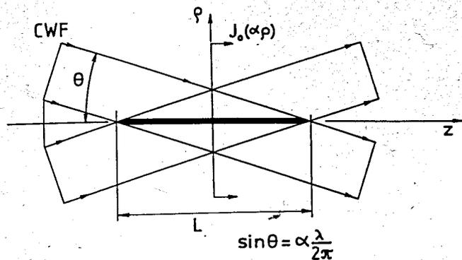
Fig. 2. The structure of the crossover in the case of the conical wave front.
