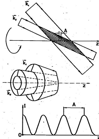
Fig. 4. Two coaxial conical wavefronts, the structure of the interference fringes and the longitudinal distribution of the light intensity on the optical axis of the system:  $\vec{k}_1$  and  $\vec{k}_2$  are two wave vectors in the given meridional cross section,  $A$  - period of the light intensity modulation.
