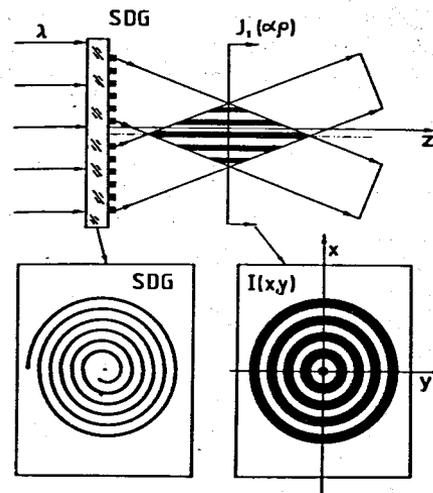
Fig. 3. The properties of the spiral diffraction grating: top - the meridional cross section of the interference fringes, bottom to the left - the view of the spiral diffraction grating, bottom to the right - the picture of the interference fringes in one of the cross sections.
