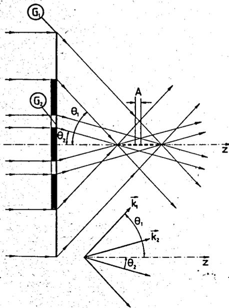
Fig.5. The experimental arrangement with two coaxial circular diffraction gratings and the wave vectors of the diffracted components:  $\theta_1$  and  $\theta_2$  are the orientation angles of the diffracted light into the plus first diffraction orders of two coaxial circular diffraction grating.
