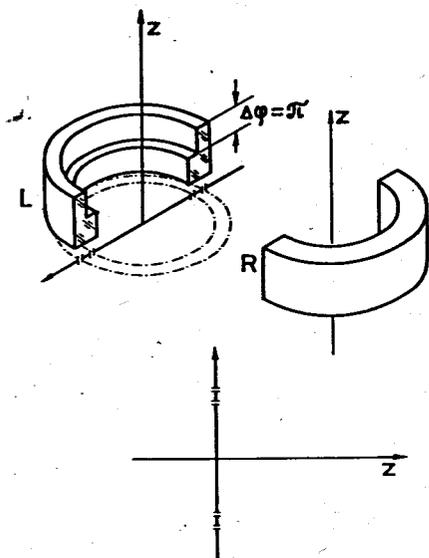
Fig. 8. The view of two halves of the ring phase jump filter with  $\Delta\phi = 180^\circ$  (see text).
