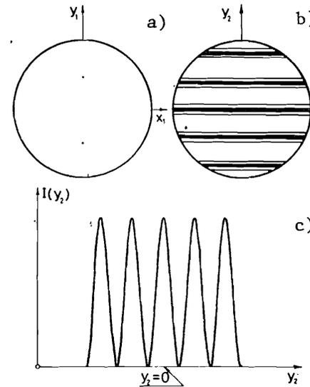
Fig. 4. a) The object plane ( $x_1, y_1$ ) with two silver grains. b) The picture of the light intensity distribution for this object in the Fourier plane ( $x_2, y_2$ ) of the MFTM. c) The curve of the light intensity distribution versus  $y_2$  at  $x_2 = 0$ .
