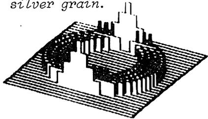
Fig. 3. 3D-plot of 2D-light intensity distribution at the exit plane of the MFTM for a particle track of four silver grains.
