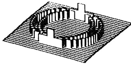
Fig. 2. 3D-plot of 2D-light intensity distribution at the exit plane of the MFTM for an object of two silver grains.
