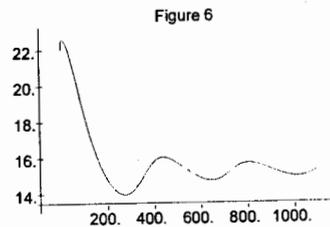
The figure 5 indicates the quantity of moisture in the wall for different time values according to the formula (27). The figure 6 indicates the mean-time value of the quantity of the moisture that was calculated according to the formula (28).
