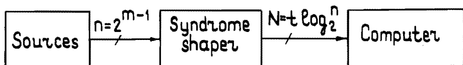
Fig. 1. Block-diagram of the data transfer system using the method of syndrome coding.
