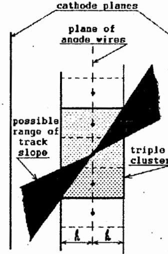
Figure 5: Schematic view of MPWC fragment.
