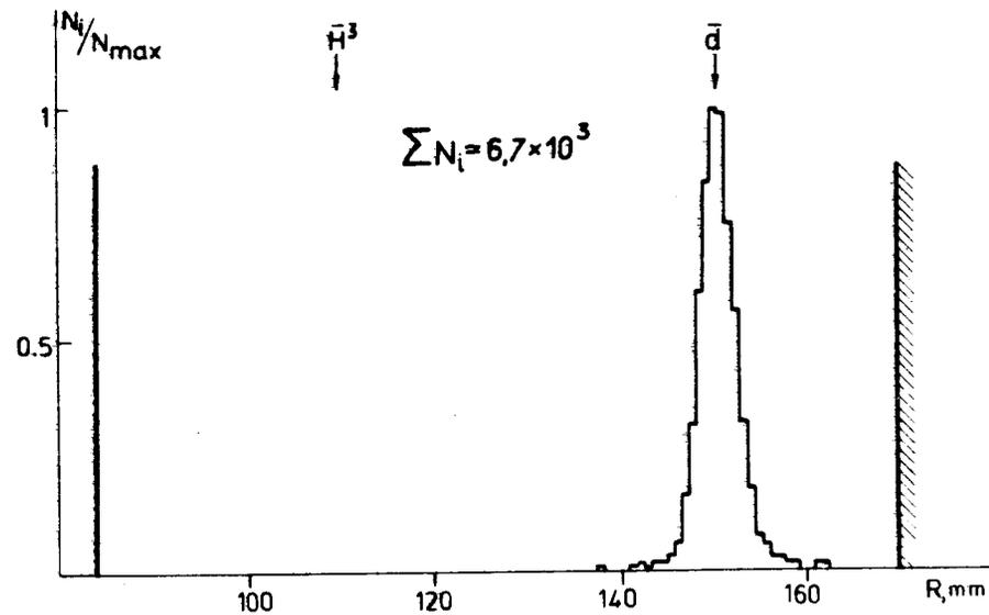
Fig. 4. Cherenkov ring spectrum for  $\overline{MC}_1\overline{C}_3$  events in MCC. The shaded lines are the boundaries of measurement ranges from blinds in front of the cathodes of the MCC photo-multipliers.
