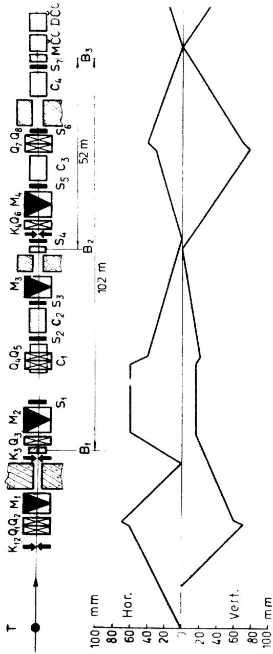
Fig. 1. Layout of the detectors in the 4B beam channel and the computed beam profile. T is the accelerator internal target, K are collimators, Q are quadrupoles, M are bending magnets, S are scintillation counters, C are threshold Cherenkov counters, B are time-of-flight counters, MCC is the multi-channel Cherenkov counter; DCC is the differential Cherenkov counter.
