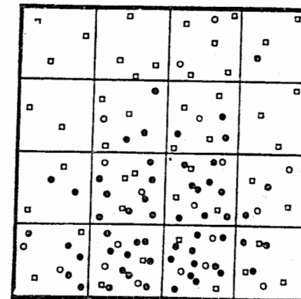
Fig.5. The area distribution of the "through-tracks" (as shown in fig.2) stopped within approximately 60 mm depth into the stack F. The area is of a size of (4 \times 4) \text{ cm}^2 . The track density decreases with increasing angle, given the angle with respect to the incident beam axis. The filled circles correspond to oxygen ions, open circles correspond to carbon ions and open squares correspond to nitrogen ions. The bottom of this figure corresponds to 20^\circ , the top to 30^\circ with respect to the beam direction.
