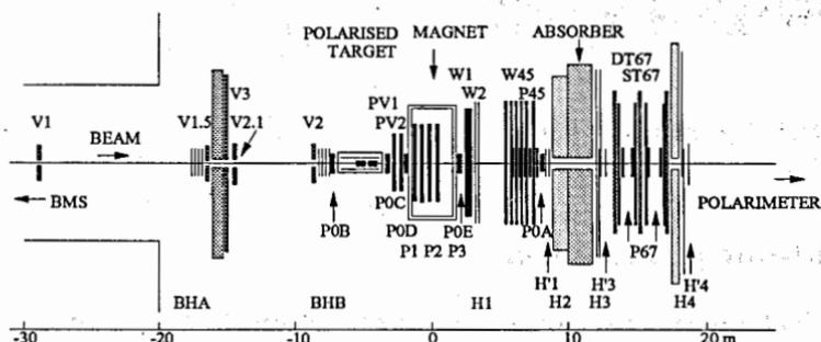
Fig.1 The Spin Muon collaboration spectrometer.
