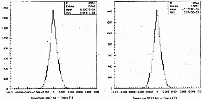
Fig. 4. Residuals between the DT67 muon line and the hits used for the fit.
