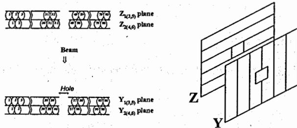
Fig. 2. DT67 geometry of planes.
