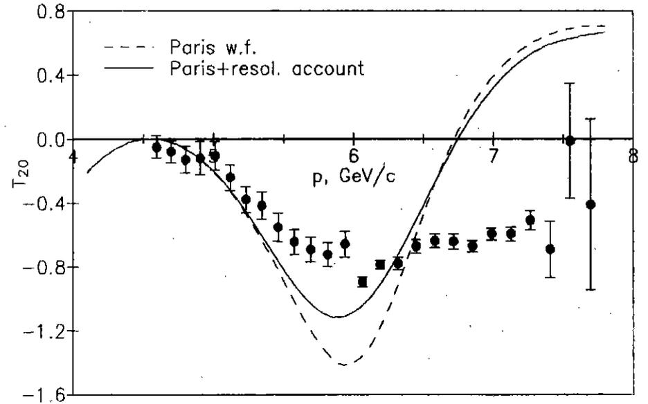
Fig. 5. Tensor analyzing power  $T_{20}$  of the reaction  $dp \rightarrow pX$  for the 9.1 GeV/c polarized deuterons and proton emission angle of  $0^\circ$  versus momentum of detected proton. The experimental data are taken from ref. [2]. The curves are calculated for the Paris deuteron wave function without reference to (dash curve) and with allowance for (solid curve) the angular and momentum acceptances of the experimental setup.
