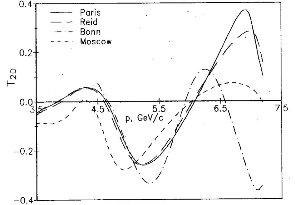
Fig. 2. Tensor analyzing power  $T_{20}$  of the reaction  $dp \rightarrow pX$  for the  $9 \text{ GeV}/c$  polarized deuterons and proton emission angle of  $139 \text{ mrad}$  versus momentum of the detected proton, calculated for the deuteron wave functions corresponding to the Paris [17] (solid curve), Reid soft core [18] (long dash curve), Bonn [19] (dot dash curve), and Moscow [20] (short dash curve) potentials of  $N - N$  scattering.
