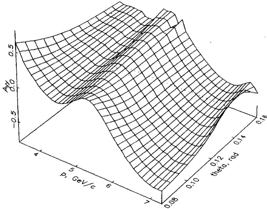
Fig. 4. Tensor analyzing power  $A_{yy}$  of the reaction  $dp \rightarrow pX$  for the 9 GeV/c polarized deuterons versus momentum  $p$  and emission angle  $\theta$  of detected protons. The deuteron wave function for the Paris potential was used.
