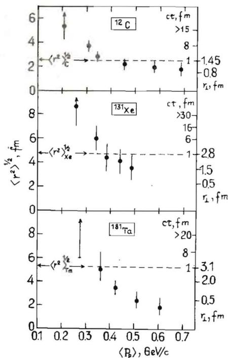
Let us consider the scales in Fig. 1. The scale on the left-hand side shows the RMS radii of the proton emission volumes extracted from the data. In order to determine these values, the experimental correlation functions have been compared with the theoretical ones containing the radius  $r_0$  of the emission volume and the lifetime  $\tau_0$  of the sources as free parameters<sup>3, 27/</sup>. In the theoretical description the emission points were assumed to be independent
