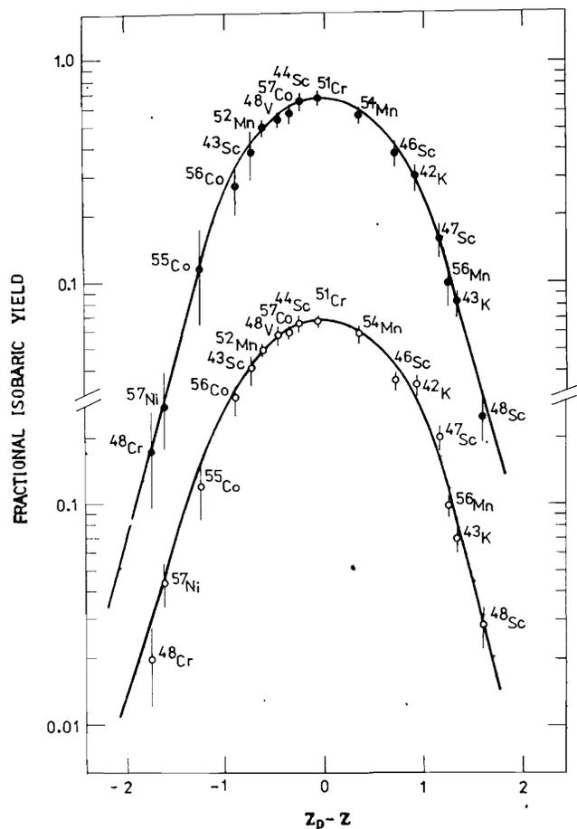
Fig. 1. Charge-dispersion curves for products over a mass range of  $42 \leq A \leq 57$  from the spallation of nickel by 9 GeV/c protons and deuterons. The upper curve and filled points are for deuterons, the lower curve and open points are for protons. Both curves are displayed vertically by a factor of 10 for display purposes.
