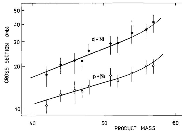
Fig. 2. Mass-yield curves for products in a mass range of  $42 \leq A \leq 57$  from the spallation of nickel by 9 GeV/c protons and deuterons.
