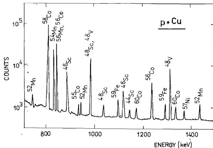
Fig. 1. Portion of a gamma-ray spectrum of a copper target recorded 1.5 day after proton irradiation. Nuclidic assignments of identified gamma-rays are indicated.
