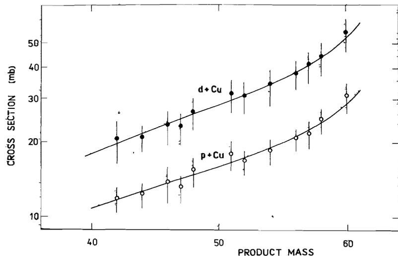
Fig.3. Mass-yield curves for products in a mass region of  $42 \leq A \leq 60$  from the spallation of Cu by 9 GeV/c protons and deuterons. The points are the sums of experimentally determined yields with estimates of missing yields from the fitting procedure described in the text.
