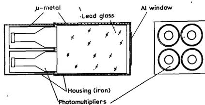
Fig.4. A schematic diagram of the Cherenkov lead-glass spectrometer. The radiator dimensions are  $18 \times 18 \times 30 \text{ cm}^3$ . The radiation length is 2.5 cm. The energy resolution,  $R$  for 4 GeV electrons is 5% (HWHM).
