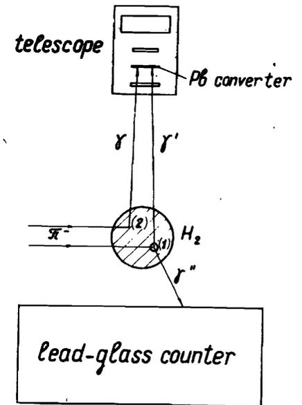
Fig.3. The Cherenkov lead-glass calorimeter (1957) used to measure the interaction cross sections between 2-10 GeV neutrons and protons, neutrons and nuclei. The Pb glass size is  $50 \times 50 \times 50$  cm<sup>3</sup>. The radiation length is 2.5 cm. The energy resolution for 1 GeV electrons is 14% (HWHM).
