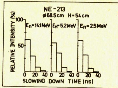
Fig. 8. Slowing-down time of neutrons in the 200 l NE-213 scintillator. The cut-off neutron energy is 0.25 MeV.
