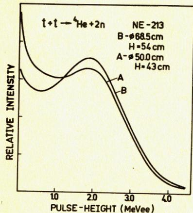
Fig. 7. Pulse-height distributions from 84 l (curve A) and 200 l (curve B) scintillators, for (t+t)-reaction neutrons.
