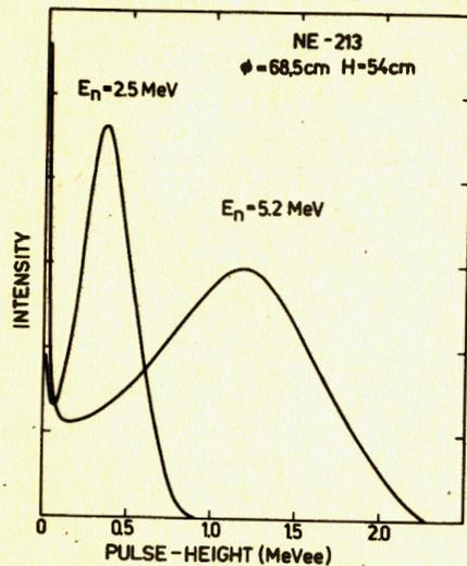
Fig. 5. Pulse-height distributions obtained for 200 l NE-213 scintillator for 2.5 MeV and 5.2 MeV neutrons.
