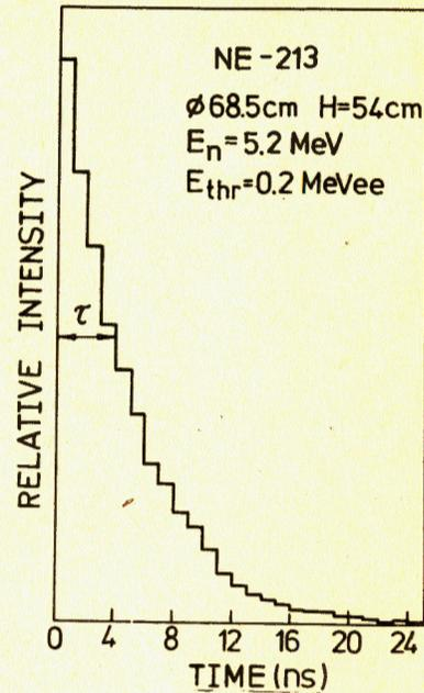
Fig. 9. Time response function of the 200 l scintillator for 5.2 MeV neutrons and for detection threshold 0.2 MeV. The time resolution  $\tau$  is marked.
