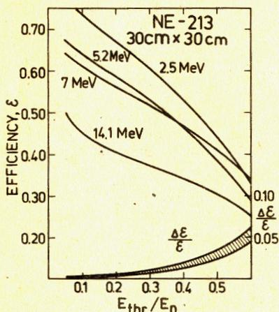
Fig. 4. Efficiency of NE-213 scintillator (30 cm diam. and 30 cm height) for different neutron energy vs relative threshold (upper curves) and relative error which arise when neglecting the light attenuation effects (lower curve).
