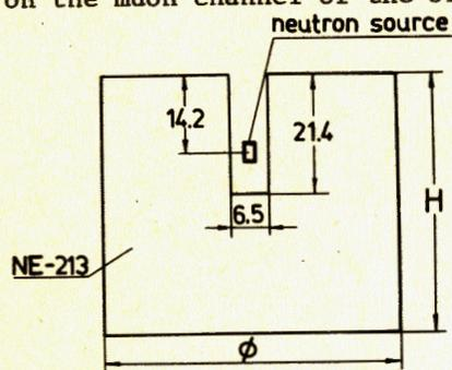
Fig.1. The sketch of the scintillator geometry.
