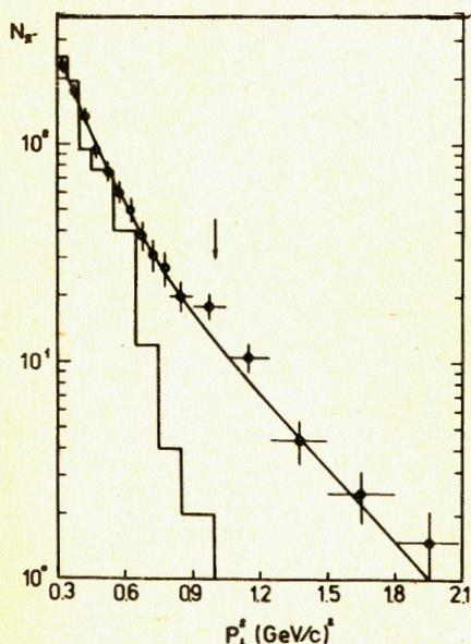
Fig. 5. Inclusive  $\pi^-$  meson  $P_{\perp}^2$  distribution summed up for d,  ${}^4\text{He}$ , C interactions with carbon and tantalum with  $P_{\perp}^2 \geq 0.3$  (GeV/c) $^2$ . The histogram shows the result of the DCM calculations.
