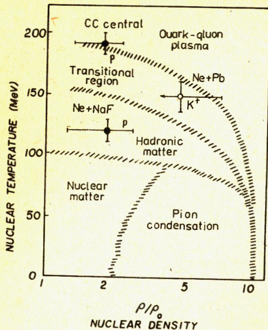
Fig.9. Theoretical boundaries for possible phase transitions of nuclear matter on the temperature-density plot. The result obtained for central collisions is shown along with the results of Refs. /61-63/ at lower energies.
