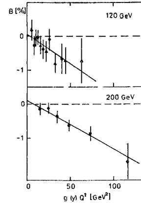
Fig. 3. The measured B asymmetry after radiative corrections at 120 GeV and 200 GeV beam energy vs.  $g(y)Q^2 = Q^2 \cdot [1 - (1-y)^2] / [1 + (1-y)^2]$  [eq. (3)]. For the 120 GeV data, circles represent data with  $Q^2 > 5 \text{ GeV}^2$  and triangles data with  $Q^2 > 25 \text{ GeV}^2$ . Solid lines are straight line fits to the data.
