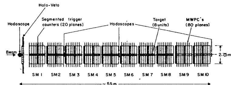
Fig. 1. Schematic layout of the experimental set-up.
