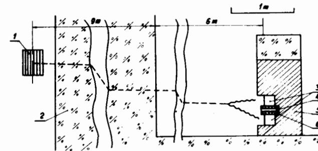
Fig.1. Schematic diagramme of the installation. 1 - reactor core, 2 - reactor shielding, 3 - scintillation counters, 4 - anticoincidence counter, 5 - iron shielding, 6 - lead.
