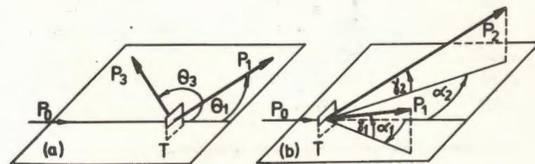
Fig.1. Geometric conditions of the measurements.  $p_0$  - incoming proton beam,  $T$  - target. (a) coplanar geometry of  $p_1$ - $p_3$  registration, (b) noncoplanar, symmetric geometry of  $p_1$ - $p_2$  registration.
