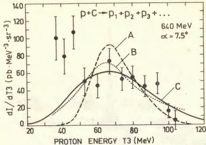
Fig. 3. Energy spectrum of backward emitted protons measured in the triple coincidence experiment. The curves represent phase space calculations for process (2) and are normalized to the experimental  $T_3$  spectrum between 52 and 104 MeV. A, without the Fermi motion of the  $[pp]$ -pair taken into account; B, with the Fermi motion; C, with the Fermi motion and the  $|T|^2$  dependence according to relation (4) with  $a_{ch}=0.3$  fm.
