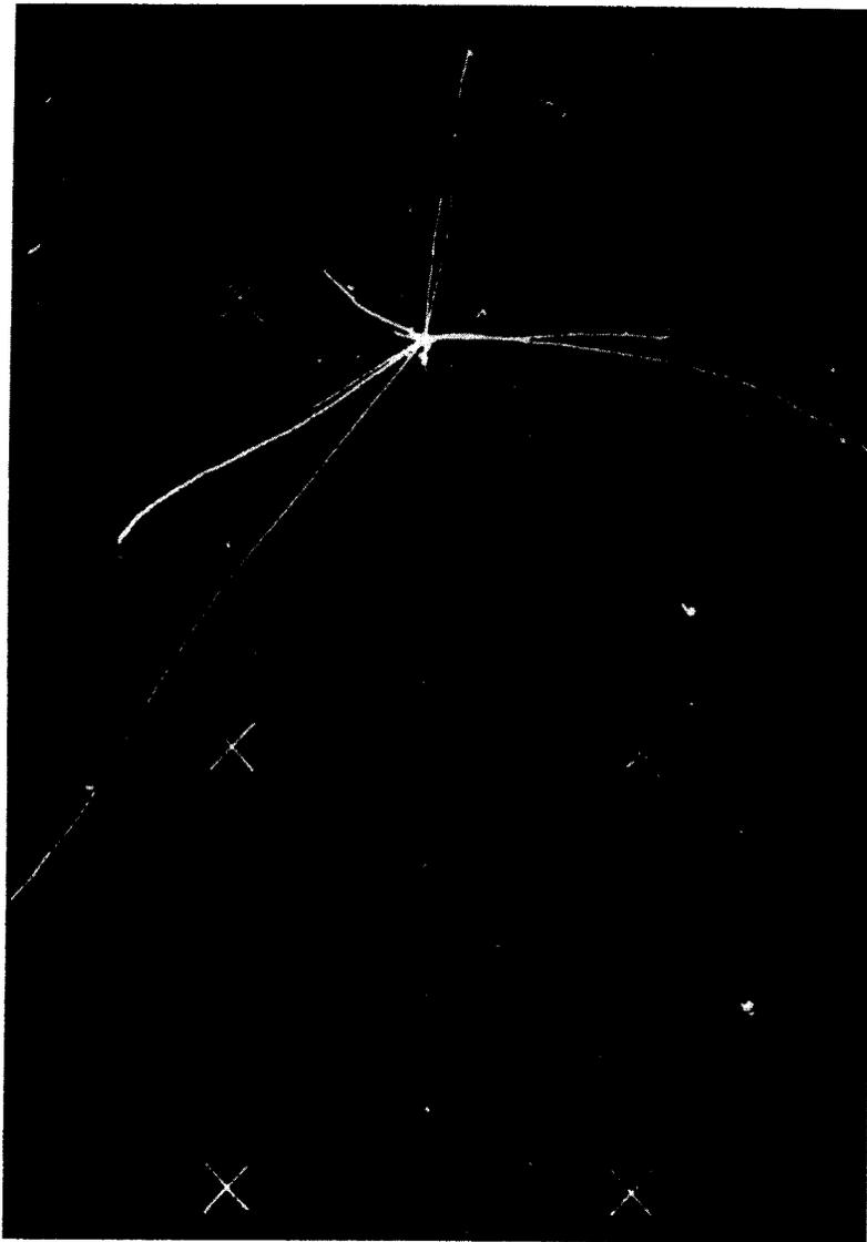
*Fig. 1. Collision of negative pion of  $3.5 \text{ GeV}/c$  momentum with xenon nucleus, not accompanied by the multiparticle production; all secondaries are protons.*
