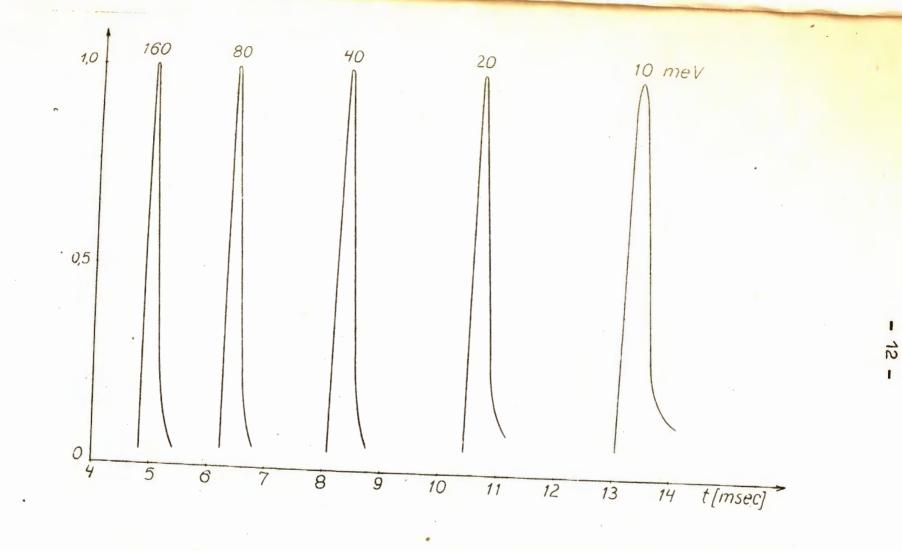
Fig. 4. Shape of resolution curves for various values of changes in energy for flight path  $L_1 = 20.2 \text{ m}$ ,  $L_2 = 1.2 \text{ m}$ , and energy  $E_r = 4.94 \text{ meV}$
