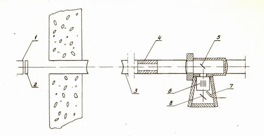
Fig. 1. Diagram of spectrometer. 1 - reactor core, 2 - moderator, 3 - vacuum tube, 4 - collimator, 5 - sample, 6 - beryllium filter with collimating cadmium inserts, 7 - tray of BF<sub>3</sub> counters, 8 - monocrystal
