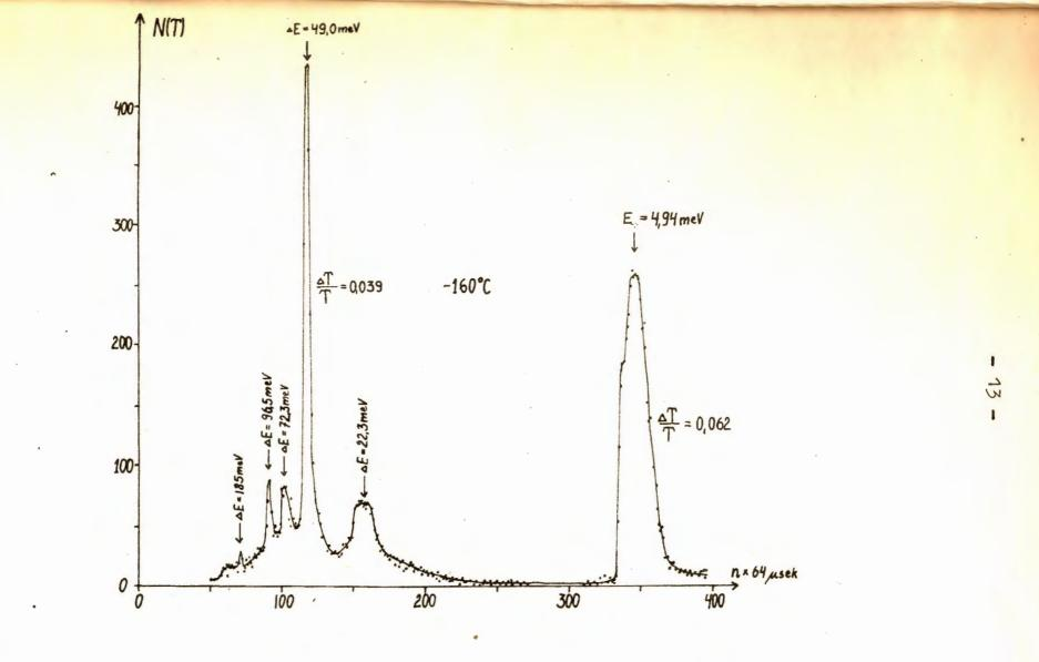
Fig. 5. Spectrum of neutrons scattered from polycrystalline ammonium chloride at a temperature of -160°C
