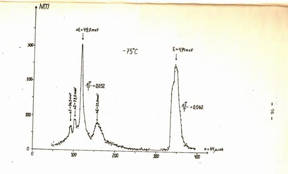
Fig. 6. Spectrum of neutrons scattered by polycrystalline ammonium chloride at a temperature of -75°C.
