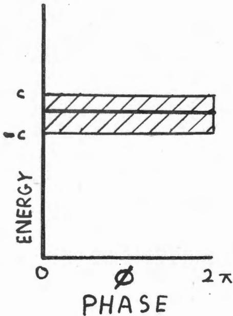
Fig. I. Initial distribution of particles in Phase Space in the stacked beam.
