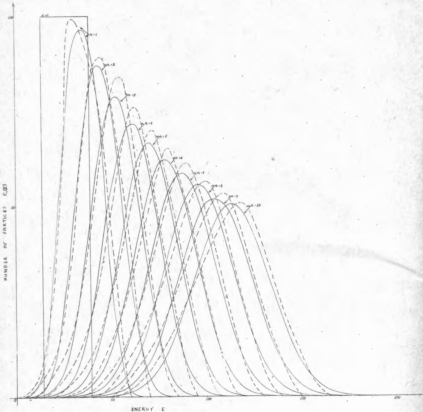
Fig. 2. Comparison of the Energy Spread in the stacked beam as predicted by Eq. (17) with Swenson's exact calculations. The different curves refer to the number  $n$  of passages of the rf bucket. The solid curves are predictions of Eq.(17), the broken lines those obtained by Swenson.
