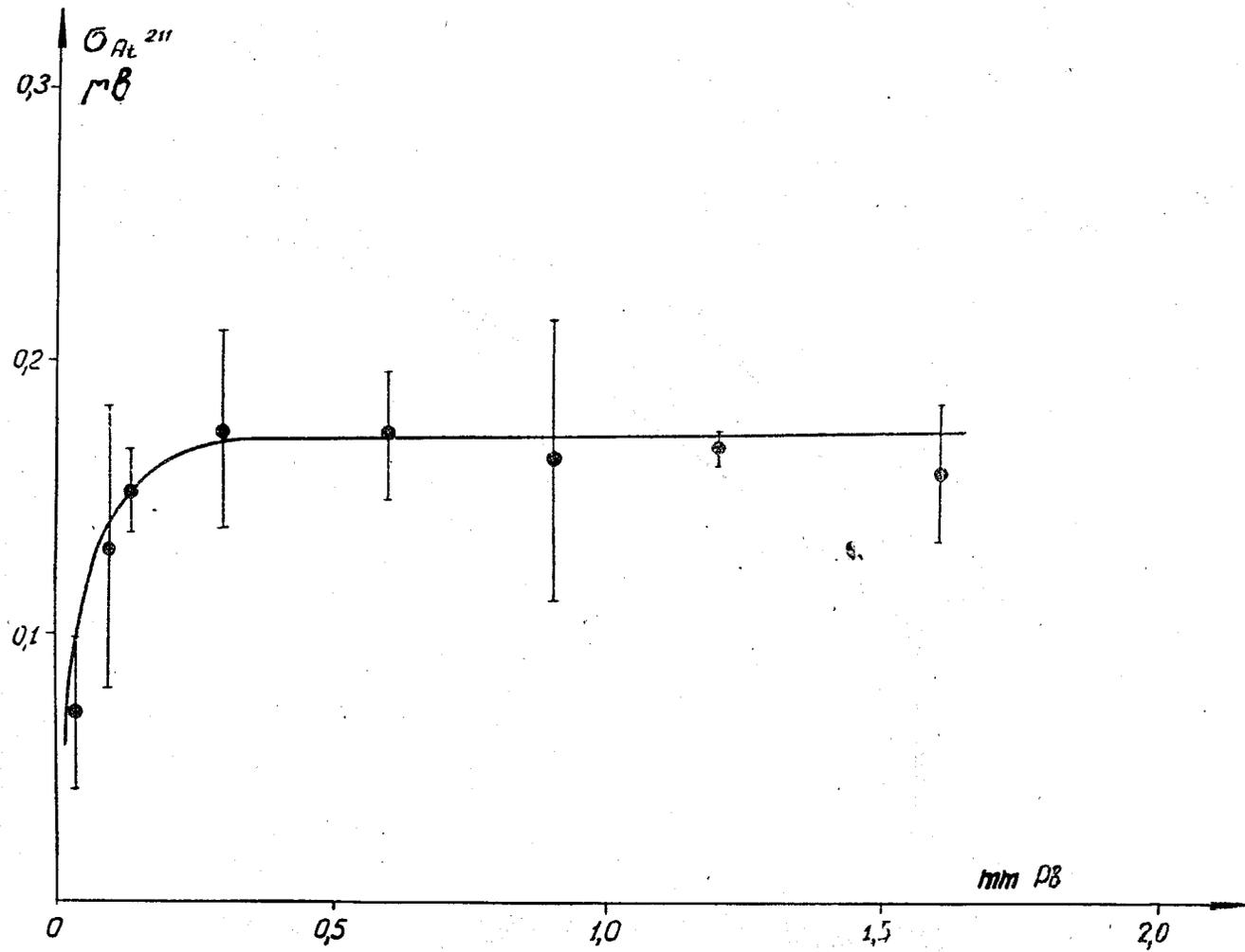
Fig. 2. The yield of the isotope  $At^{211}$  from lead foils of different thickness.
