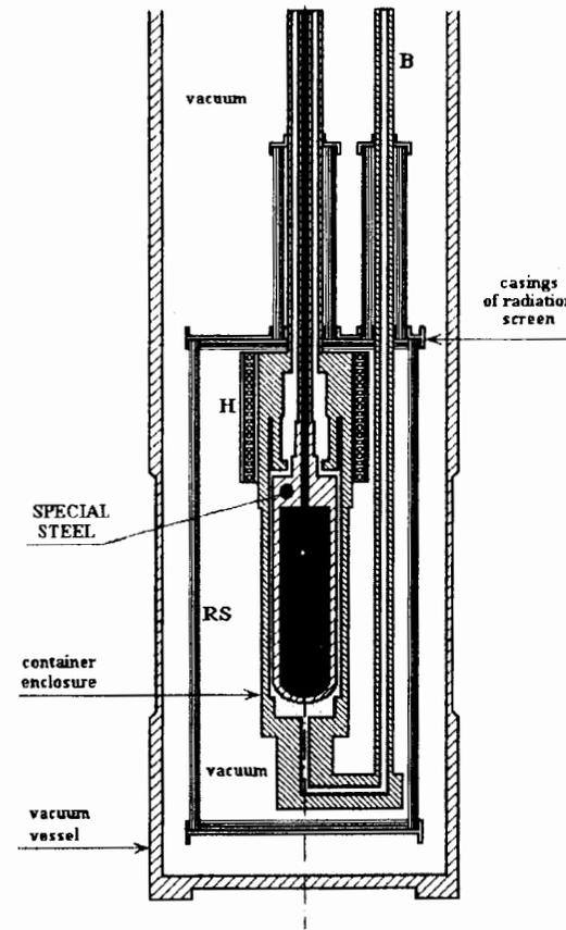
Figure 17: Schematic view of the Tritium High Pressure Target. A target container, B tube for the cooling agent (hydrogen) and the path for pumping the diffusing tritium. H heater. RS radiation screen.
