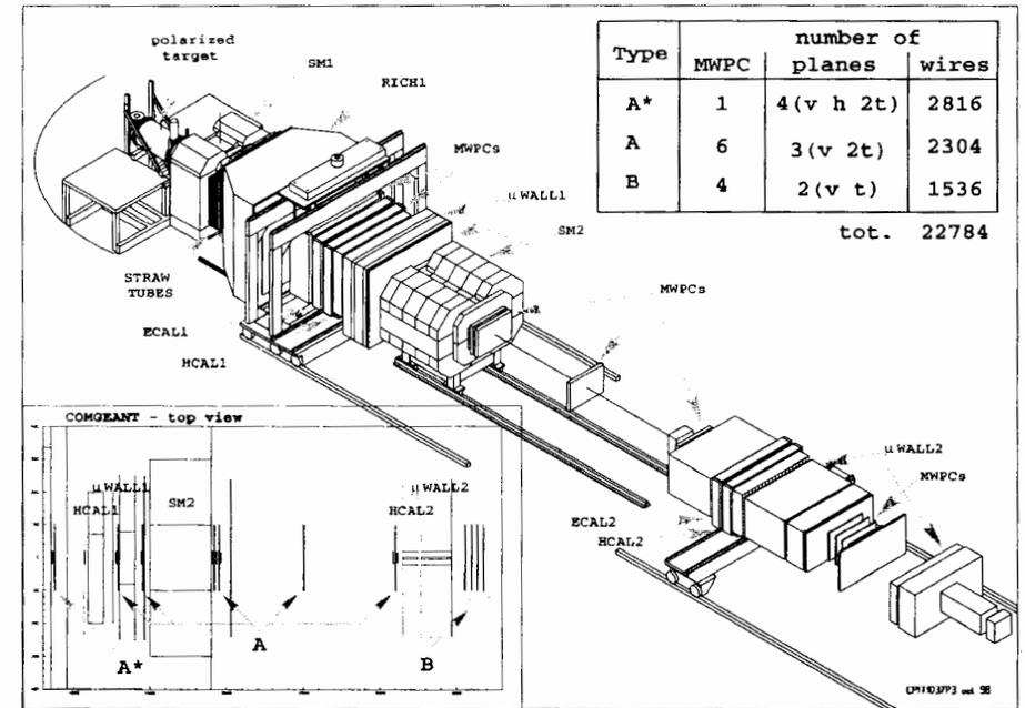
Figure 14: Multiwire proportional chambers in the COMPASS initial setup.
