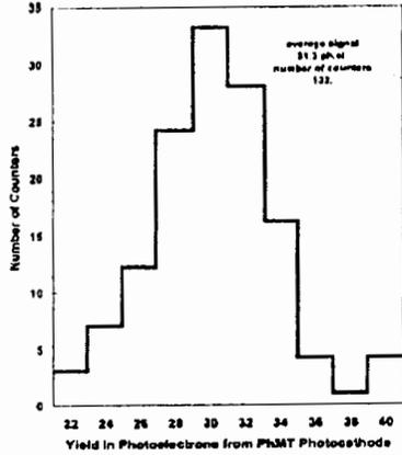
Figure 13: Yield of photoelectrons from scintillator counters for the new muon trigger of the Upgraded CDF
