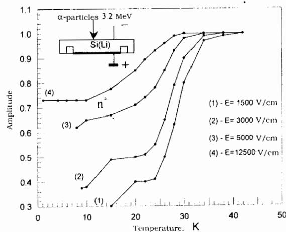
Figure 23: Signal amplitude as a function of the temperature for various bias voltages applied to the detector.
