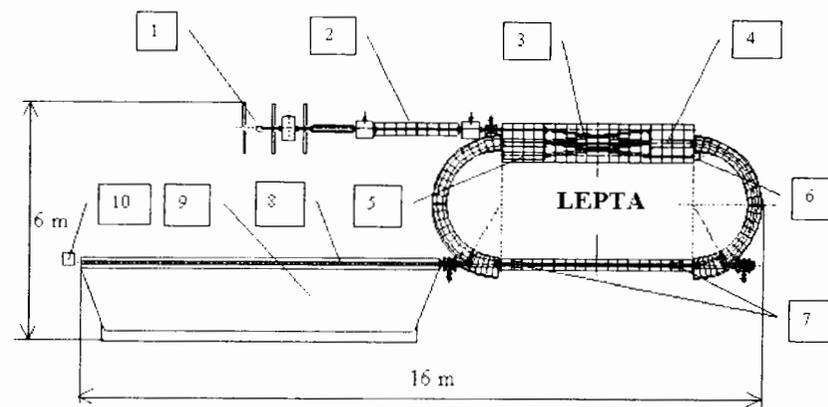
Figure 26: LEPTA layout: 1 — positron source, 2 — positron trap, 3 — septum coils, 4 — kicker, 5 — electron gun, 6 — electron collector, 7 — pick-up stations, 8 — decay channel, 9 — dipole magnet, 10 — Ps detector.
