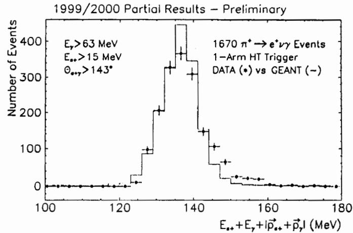
Figure 16: Pion invariant mass of the decay  $\pi \rightarrow e\nu\gamma$ .
