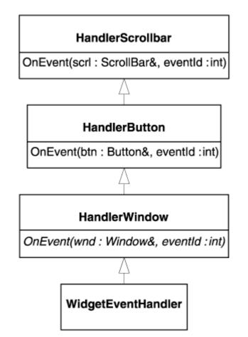
Figure 3.5. A size-optimized structure for WidgetEventHandler
