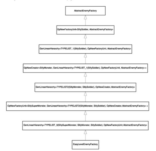
Figure 9.3. The class hierarchy generated for EasyLevelEnemyFactory
