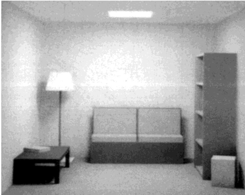
Figure 9.16: An image computed using Monte Carlo path tracing, with the radiosity solution supplying the radiance at secondary ray intersections. Courtesy of Holly E. Rushmeier, Program of Computer Graphics, Cornell University.
