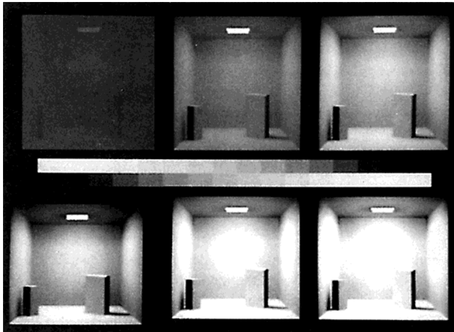
Figure 9.22. Images produced after accounting for brightnesses and viewer adaptation based on work by Tumblin and Rushmeier. Light source intensities range from 10^{-5} lamberts to 10^3 lamberts in geometrically increasing steps by 100. Courtesy of Jack Tumblin, Georgia Institute of Technology.
