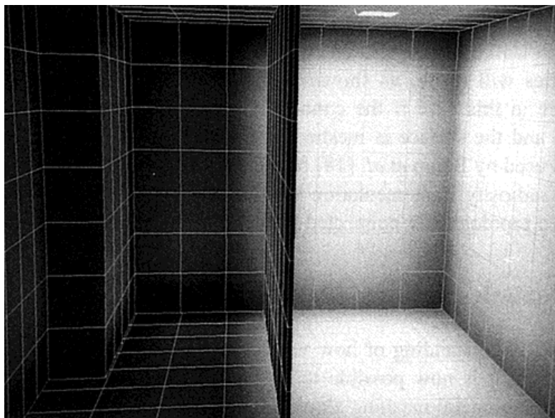
Figure 6.18: A light leak caused by failure to resolve discontinuities in value where the dividing wall touches the floor. The dividing wall completely separates the left side of the room from the right side, which contains the light source.
