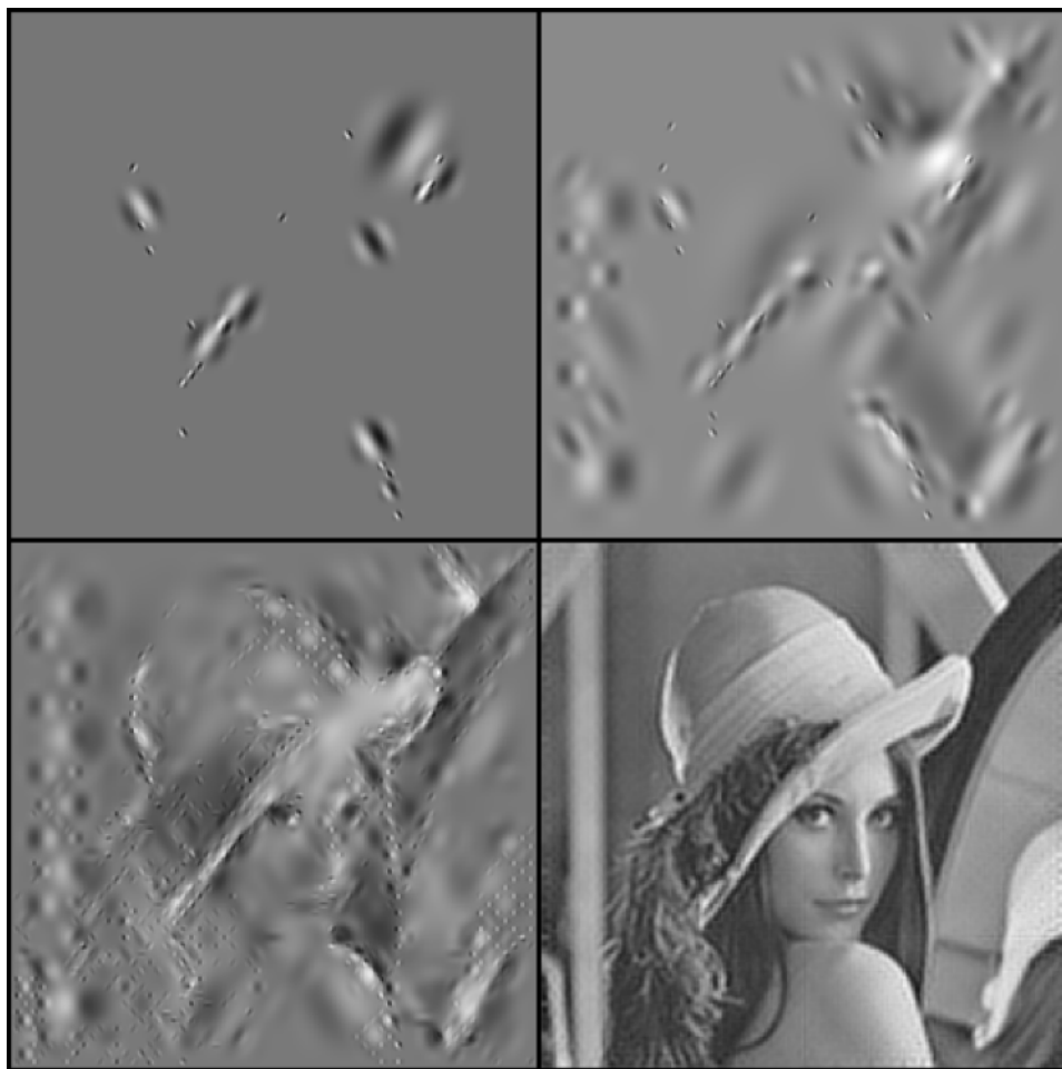
Figure 2. Illustration of the completeness of 2D Gabor wavelets as image coding primitives. The benchmark “Lena” picture is reconstructed by progressive numbers of wavelets in linear combination, of 25, 100, 500, and 10,000. The primary facial features are effectively represented by just a handful of such wavelets. However, because of their nonorthogonality, the wavelets require coefficients that differ from the simple inner product projection of the image onto them.
